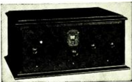
Fig. 2—Front view of the new Baird universal short-wave and television receiver, showing the extremely simple controls and the single tuning dial.
